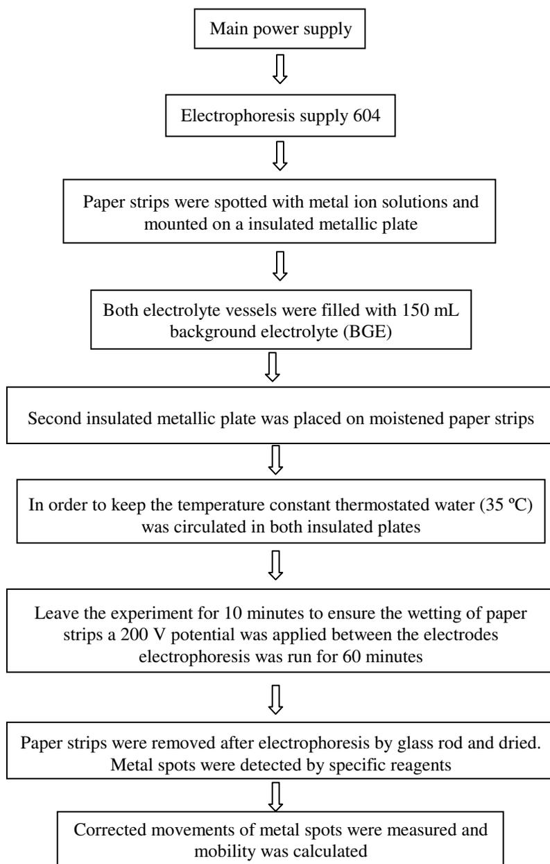
**Figure 2:** The scheme for paper electrophoresis set
