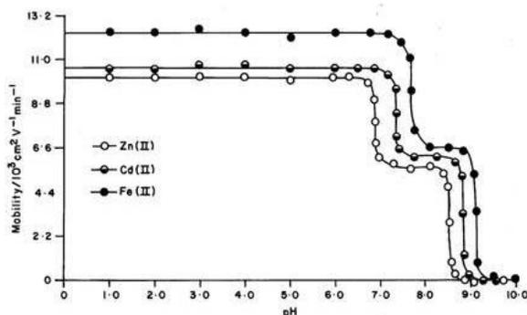
**Figure 1:** Mobility curves for the metal(II) – homoserine systems. Background electrolytes: 0.1 M perchloric acid and 0.01 M homoserine. The paper strips were spotted with 0.1  $\mu$ L of sample solution and glucose (for making osmotic correction).
